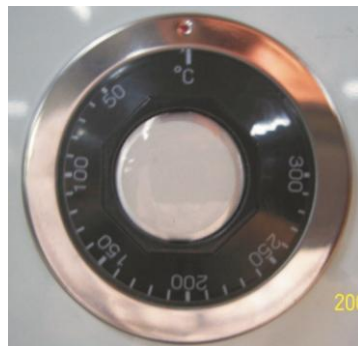
Picture 4-4: Setting the Over-thermal Protector
