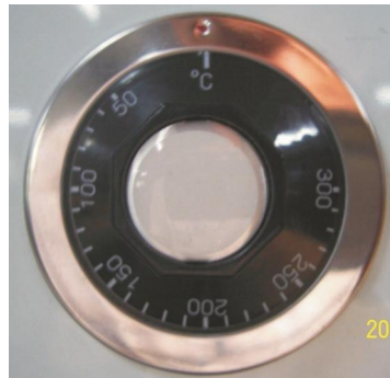
Picture 4-4: Setting the Over-thermal Protector
