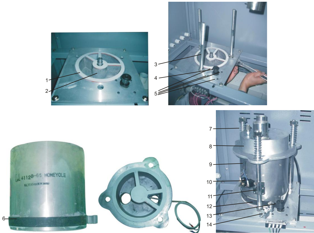
Picture 3-2: Installation of the Rotor (SD-30H~700H)
