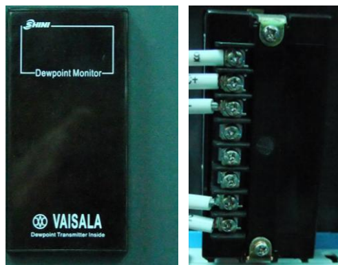
Picture 4-16: Installation for Dew-point Monitor
