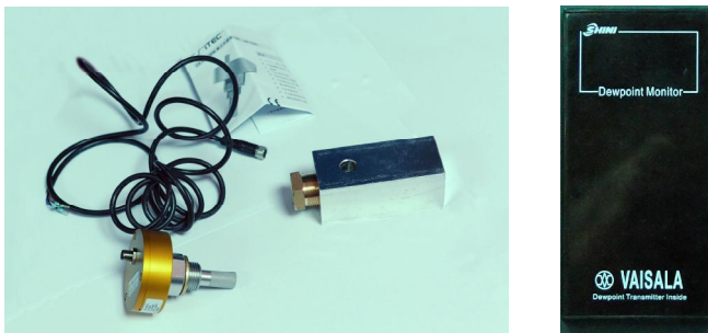
Picture 4-11: Parts of Dew-point Monitor
