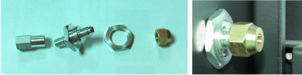
Picture 4-12: Copper Joint Assembly of Original Machine
