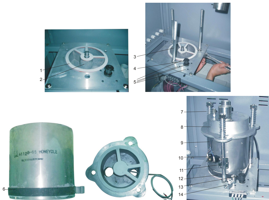
Picture 6-3: Installation of The Rotor
