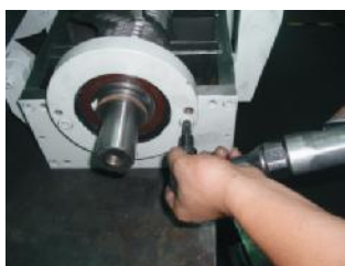
Picture 3-5: Installation of Bearing and Cutter Shaft 3
