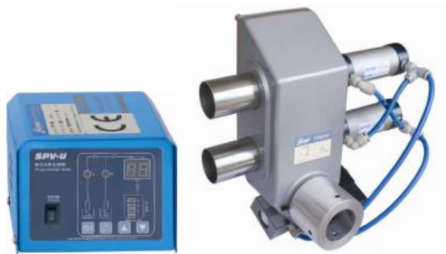
Picture 2-24: Control Cabinet and Valve
