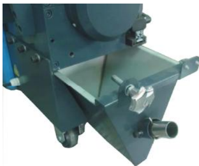
Picture 3-12: Installation of Feed Box, Feed Port and Storage Box 4
