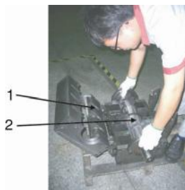
Picture 3-4: Installation of Bearing and Cutter Shaft 2
