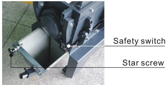
Picture 2-2: Safety Switch
