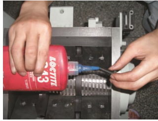
Picture 6-1: Blades Maintenance
