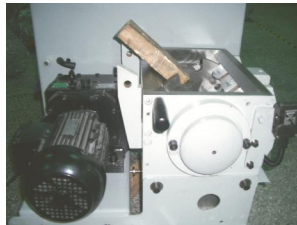
Picture 6-2: Dismantle Fixed Blades
