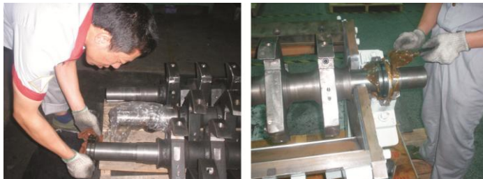
Picture 3-5: Installation of Bearing and Blade Rest
