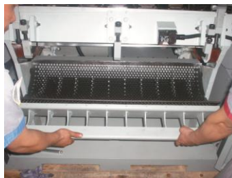
Picture 4-3: Close the screen bracket; the storage box and the feeding hopper.
