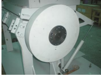
Picture 3-14: Installation of Belt Pulley and Motor 4 (SG-3675)
