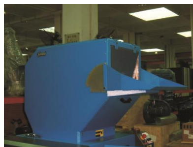
Picture 6-19: Installation of Feed Box and Feed Inletv 5
