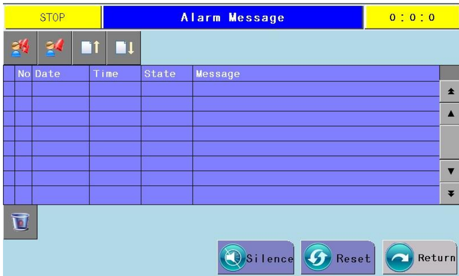
Picture 4-24: Alarm Message Interface
