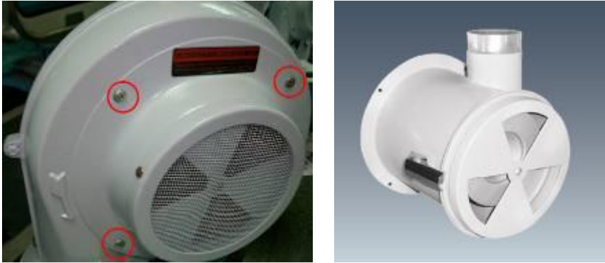
Picture 3-7: Right: AIF blower inlet filter
