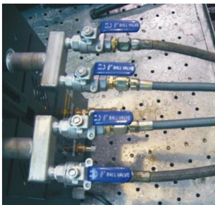
Picture 3-3: Mould and Water Coupling 2
